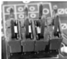
A B C D all pins installed = 1000 ppm
