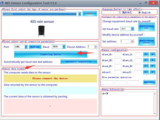
6. Then if the sensor is well connected, user can see data status on "Sensor data window"
